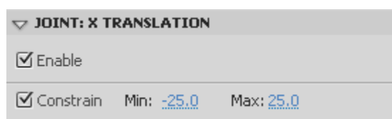
Figure 7 – Constraining Joint: X Translation
